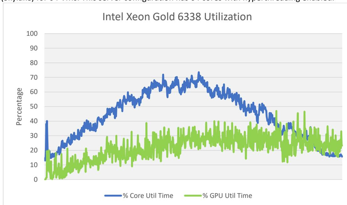
This graph of the 64 VM T4 test shows that as the GPU utilization ramps up during the nVector KW workload test, CPU Core utilization is offloaded and drops accordingly.
