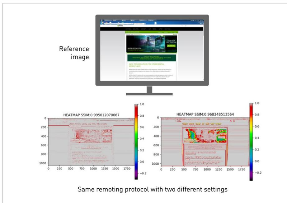
Figure 9. SSIM as a Measure of Image Quality
