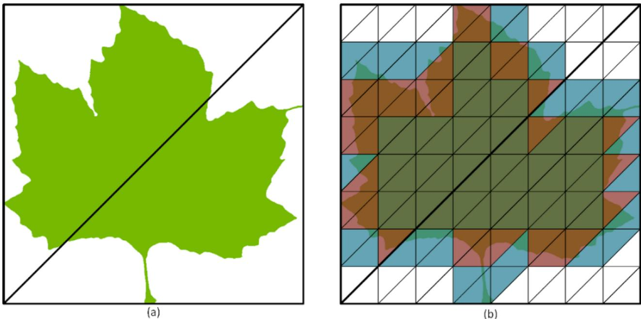
Opacity mask is applied to maple leaf which is composed of 2 triangles. The opacity engine evaluates the leaf and determines which sections are opaque, transparent, or unknown (in which case it must be sent back to the SM).
