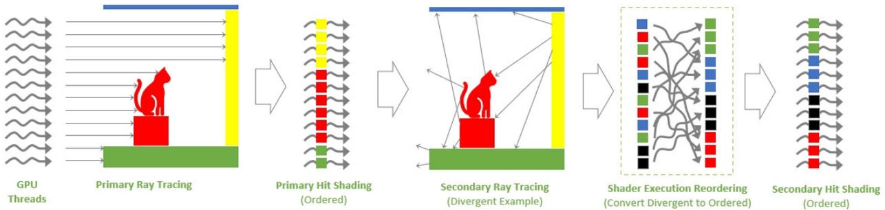
Shader Execution Reordering. Advanced lighting techniques such as path tracing cause shader divergence as secondary rays bounce off objects in the scene (denoted by various colors). In these scenarios, SER reorders shading work to improve efficiency.
